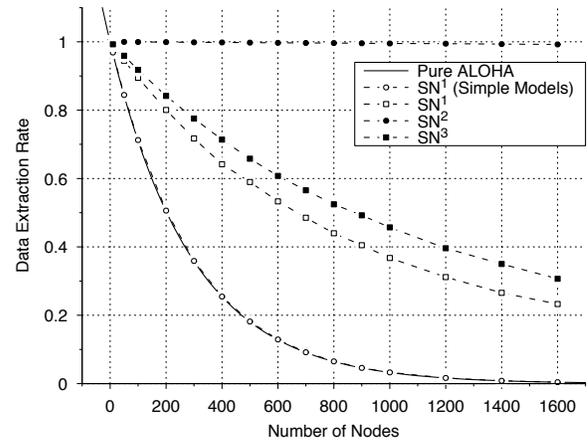
**Figure 4: Experiment Set 1 – Single Sink: Pure ALOHA and  $SN^1$  (Simple Models) overlap. As the number of nodes increases, the DER decreases exponentially. With typical LoRaWAN settings ( $SN^3$ ) and a typical  $DER > 0.9$  requirement  $N = 120$  nodes can be supported.**
