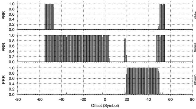
**Figure 3: Capture effect.**  $SF = 12$ ,  $BW = 250$  kHz, 55.25 symbols packet length. X-axis shows the transmission offset relative to the weak node in symbols, Y-axis shows the packet reception rate.
