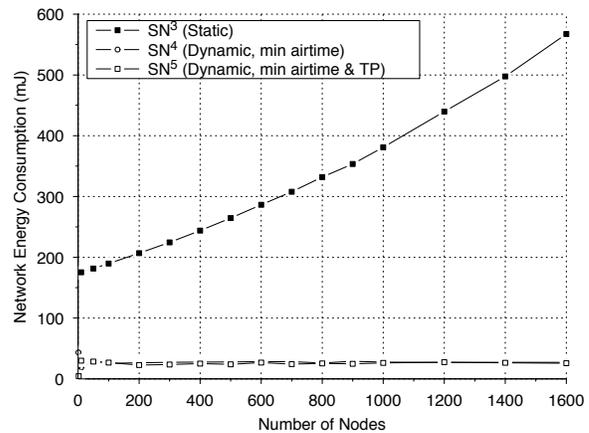
**Figure 6: Experiment Set 2 – Dynamic Parameters:** Lines for  $SN^4$  and  $SN^5$  overlap. Choosing communication parameters of nodes to minimise airtime (or airtime and power) has a significant impact on energy per extracted packet.
